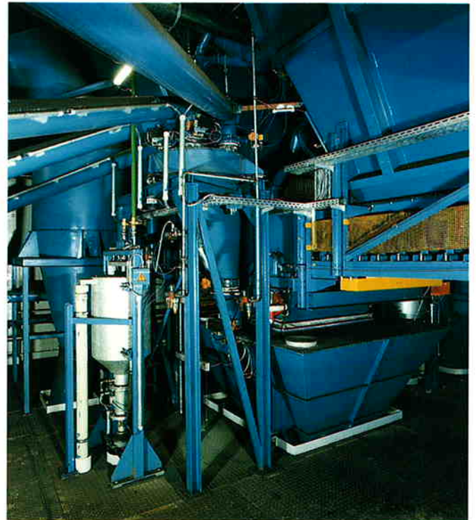
Fig. 13.3: Complete scale assembly with additives scale, water scale and metering units
