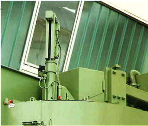
Fig.11.1: Retractable moisture sensor
