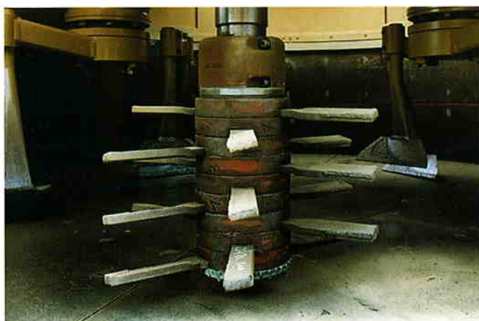
Fig.10.1: Replaceable mixing blades
