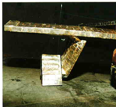
Fig.10.2: Hard metal plating
