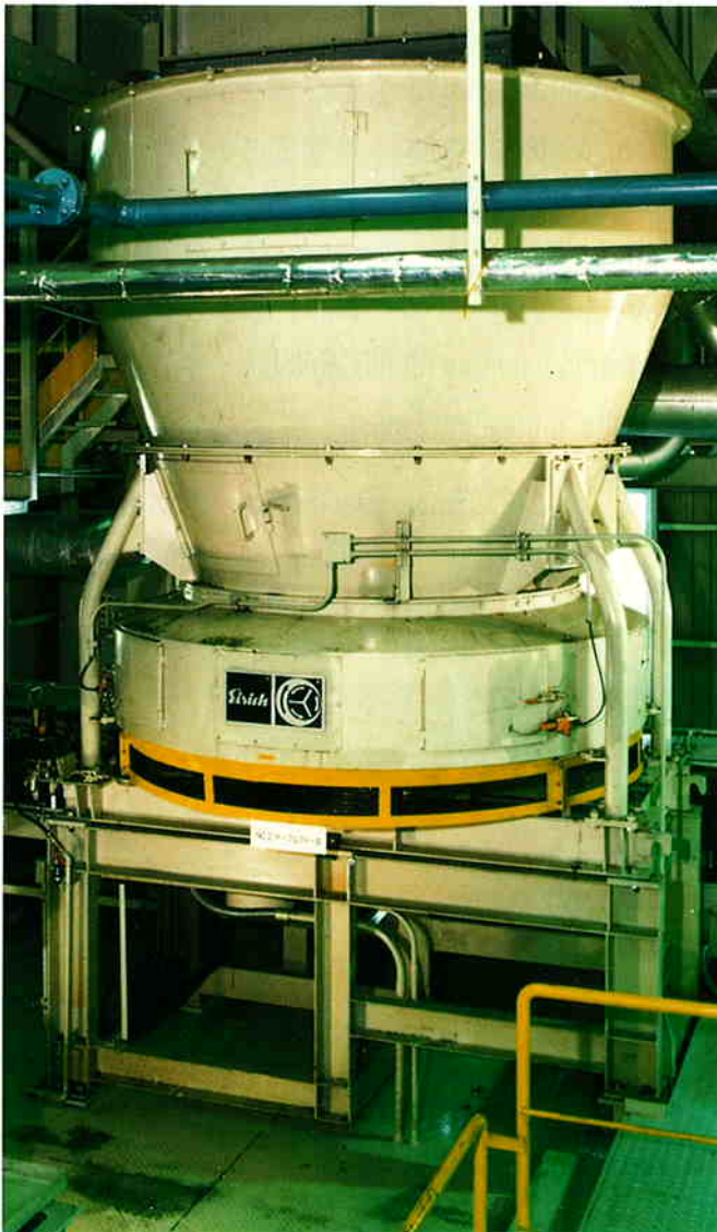
Fig.12.1: Metering unit for granular-flow materials
