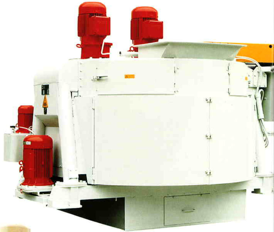
Fig.8.1: EIRICH intensive-action mixer Type D 29
